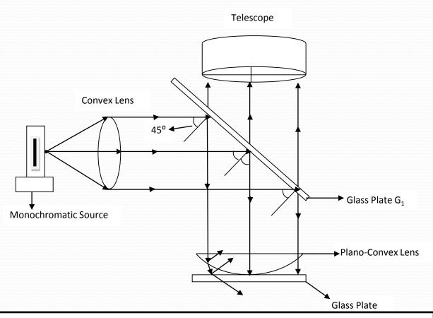
If **S** be the source of monochromatic light. When light from the source (S) is allowed to fall on a convex lens, then it render's a parallel beam of light .This parallel beam of light is allowed to fall on plane glass plate. That is placed at an angle to the direction of incident beam of light. Then the glass plate reflects the incident beam of light normally towards the air film enclosed between the Plano convex lens and the glass plate.
